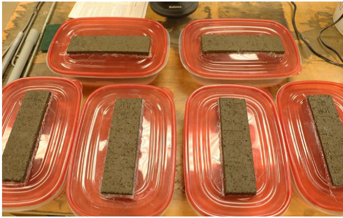
Photo 3: Brick Units Partially Submerged in Water (top left) and Hydrochloric Acid (top right)
